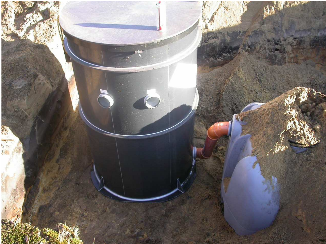
Photo 1: left : BioKube Venus 1850 (5 PE) set up in Certipro ® test facility right : pre-settlement tank (septic tank) left : BioKube Venus 1850 (5 PE)
